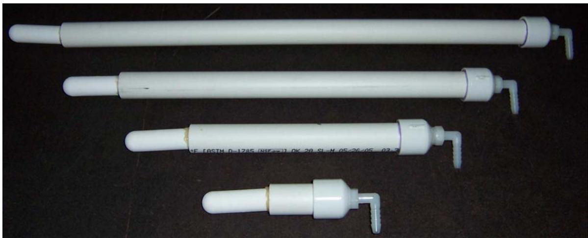
Figure 1. Lysimeters used to collect irrigation and swine effluent samples from subsurface irrigation systems at Oklahoma Panhandle Research and Extension Center.
