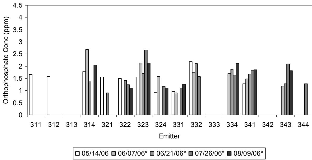
Figure 2 Orthophosphate concentrations (ppm) at the inlet end of field with a 0.19 gal hr<sup>-1</sup> emitter application rate. Background samples (05/14/06) were taken prior to annual effluent applications and soil solutions were sampled following each of the four effluent applications. Missing samples are due to inadequate sample volume collected for analysis.
