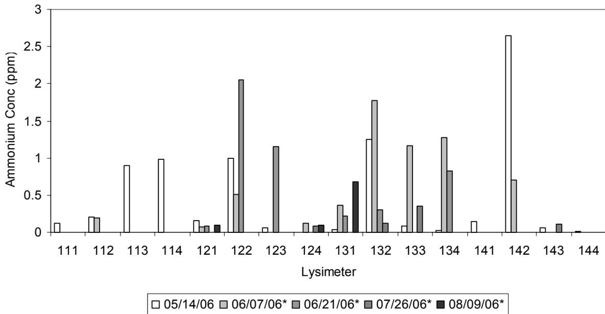
Figure 4 Ammonium-N concentrations (ppm) at the inlet end of field with a 0.63 gal hr<sup>-1</sup> emitter application rate. Background samples (05/14/06) were taken prior to annual effluent applications and soil solutions were sampled following each of the four effluent applications. Missing samples are due to inadequate sample volume collected for analysis.
