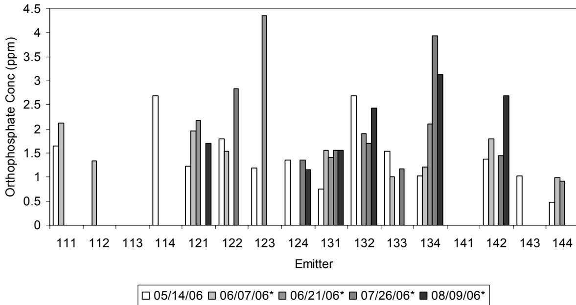
Figure 1 Orthophosphate concentrations (ppm) at the inlet end of field with a 0.63 gal hr<sup>-1</sup> emitter application rate. Background samples (05/14/06) were taken prior to annual effluent applications and soil solutions were sampled following each of the four effluent applications. Missing samples are due to inadequate sample volume collected for analysis.
