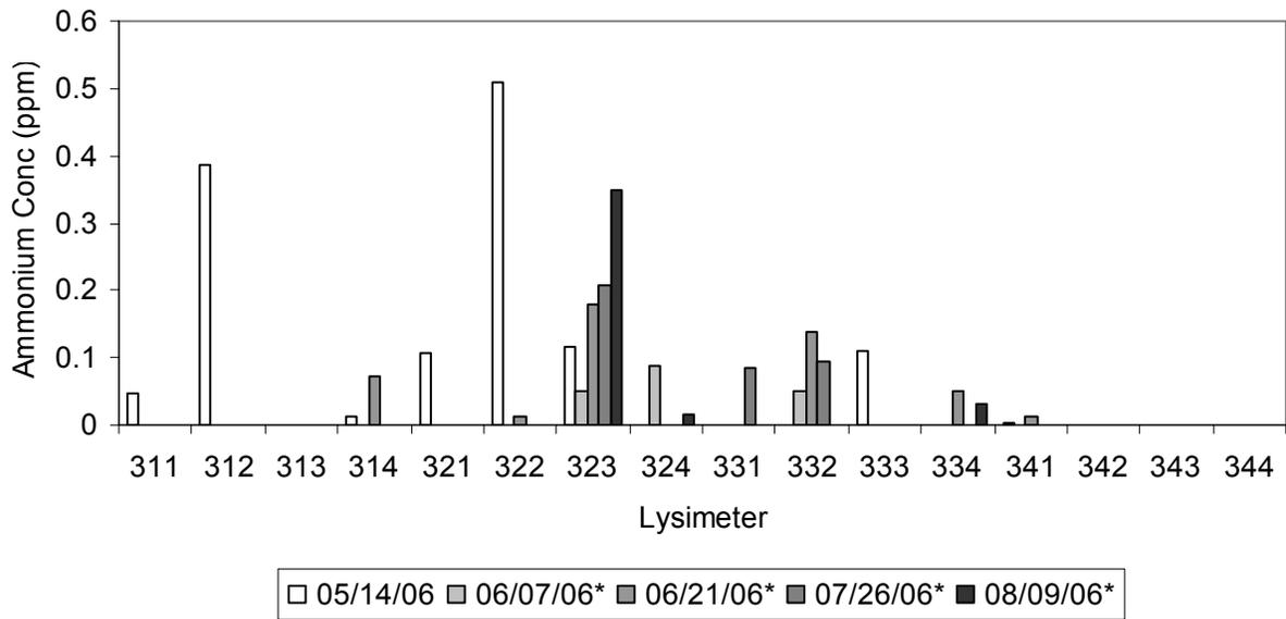
Figure 6 Ammonium-N concentrations (ppm) at the inlet end of field with a 0.19 gal hr<sup>-1</sup> emitter application rate. Background samples (05/14/06) were taken prior to annual effluent applications and soil solutions were sampled following each of the four effluent applications. Missing samples are due to inadequate sample volume collected for analysis.
