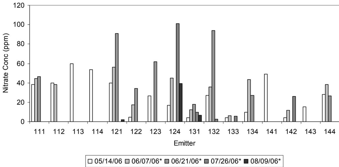
Figure 3 Nitrate-N concentrations (ppm) at the inlet end of field with a 0.63 gal hr<sup>-1</sup> emitter application rate. Background samples (05/14/06) were taken prior to annual effluent applications and soil solutions were sampled following each of the four effluent applications. Missing samples are due to inadequate sample volume collected for analysis.
