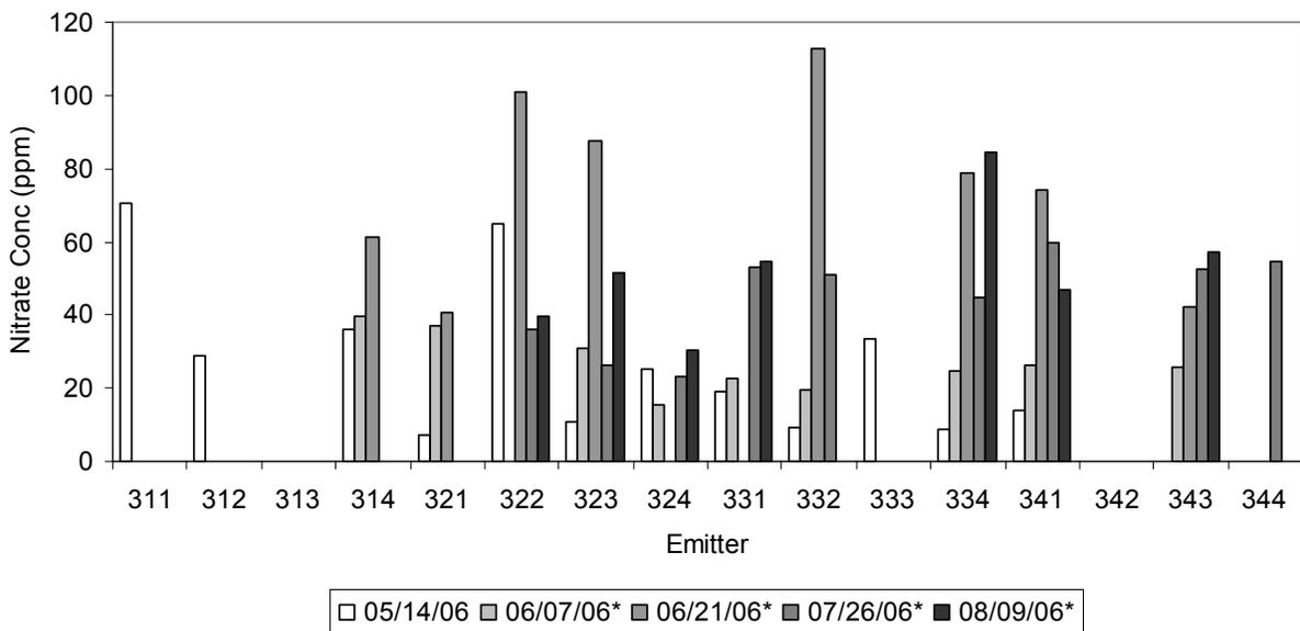
Figure 5 Nitrate-N concentrations (ppm) at the inlet end of field with a 0.19 gal hr<sup>-1</sup> emitter application rate. Background samples (05/14/06) were taken prior to annual effluent applications and soil solutions were sampled following each of the four effluent applications. Missing samples are due to inadequate sample volume collected for analysis.
