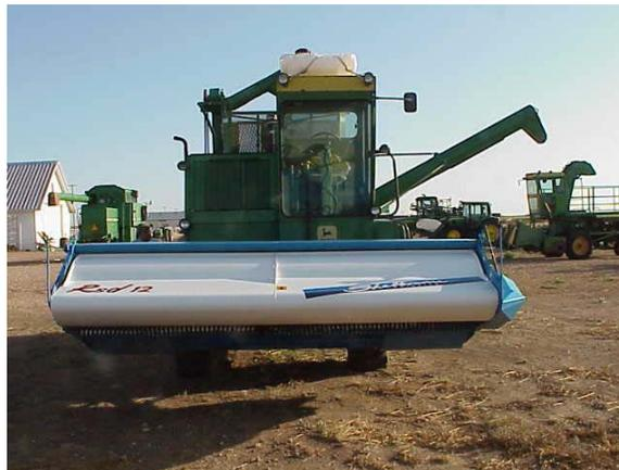
Figure 1. John Deere 3300 combine with a Shelbourne Reynolds stripper header.
