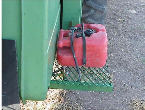
Figure 2. Auxiliary fuel tank with selector valve to enable fuel use measurement.
