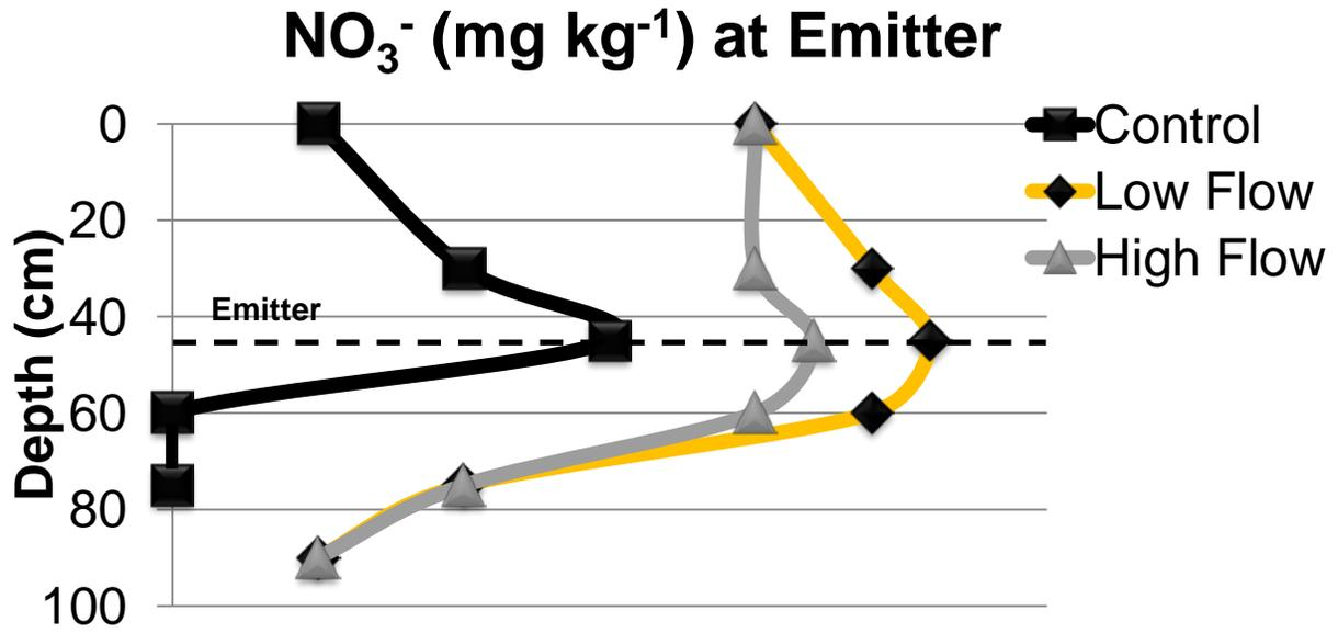
**Figure 2.** Data shows that NO<sub>3</sub><sup>-</sup> concentrations directly at emitter are higher for the Low Flow. This build up of nutrients in the low flow emitter is due to the low amount of pressure used to exert the nutrients away from the emitter and into the surrounding soil. Boron and SO<sub>4</sub><sup>-</sup> distributions were similar to the nitrate distributions as stated in Table 1.
