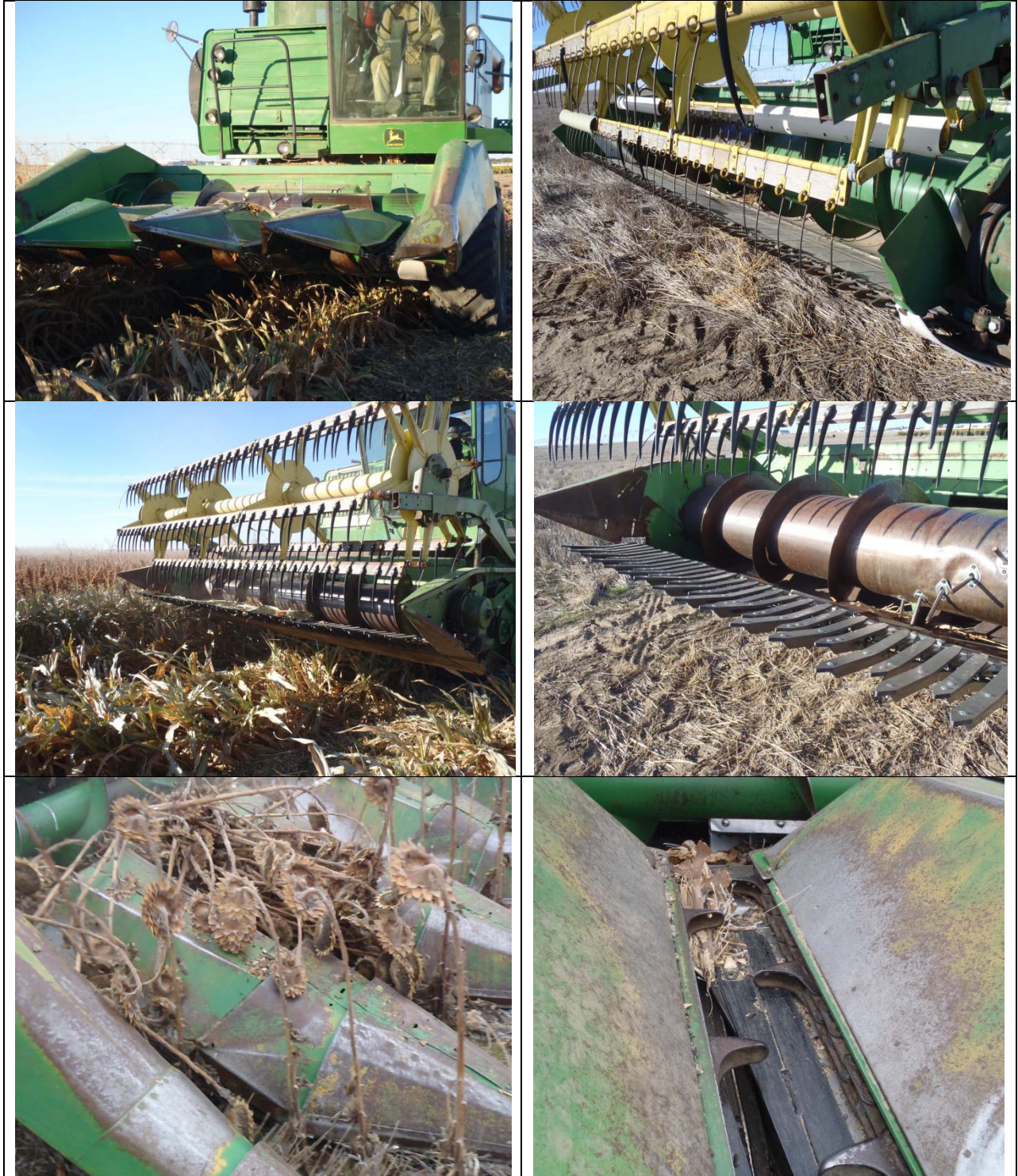
Figure 1. From top left, clockwise: Row crop head, flex bean header, conventional wheat head with Downer Milo Guards, SunStar sunflower plates for a corn header, corn header with sunflower plates and conventional wheat head (without attachments).
