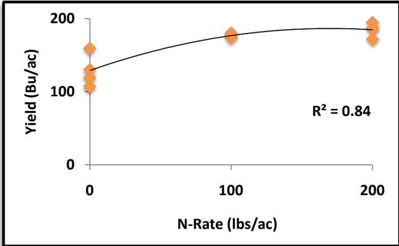
Figure 1. Nitrogen rate and final yield from the GreenSeeker™ corn trial. Grain yield was maximized between 100 and 200 lbs N ac<sup>-1</sup>.
