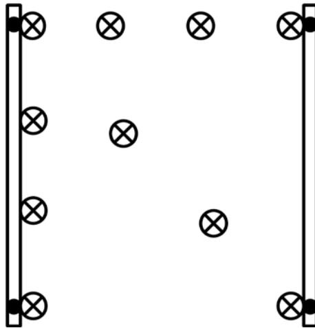
**Figure 1.** Soil Sampling Schematic. Each circle with an “X” indicates a soil core with a depth from 0-90 centimeters (cm) which were not randomly assigned for each rep. Black dots represent emitters along drip tape line. Top right emitter exemplifies emitter in question.
